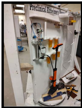
Original pneumatic system. The capacity of the reservoir was not enough.
