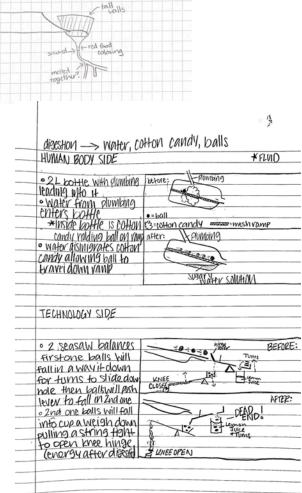
• When the balls fall into the teeter-totter it makes one side lift higher allowing the tums to fall through a hole where a cup of lemon juice is set.
