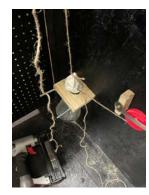
3/25/24 Today Danica, Ary and Eli worked on putting all the wiring on the back of the machine and making it look nice. We took a plastic mason jar and took the lid and drilled a hole and put a grommet in so the clear tube for the syringe wouldn't move.
