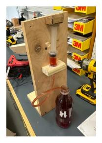
Fluid Power: We utilized both gas and liquid for this component. The first fluid power component forces a syringe to move a weight upwards which then rolls down a ramp. The second fluid power component releases the hydraulic fluid into the flask for the chemical component.
