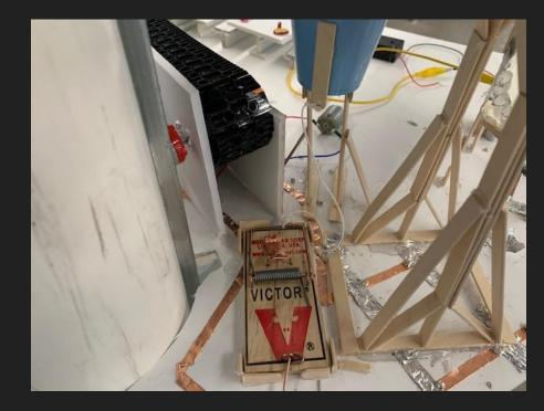
Step 8: When the mouse trap is activated, it will pull a string attached to a cup full of weight and the cup will fall off the tower.
