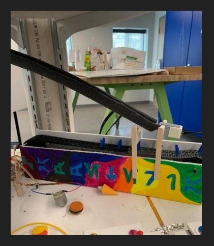
Step 7: The food will move across the conveyor belt and will drop them onto a mouse trap, making it snap.
