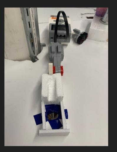
Step 5: The hole in the floor of level one has a marble ramp to guide the dropping marble down to where it hit a touch sensor.
