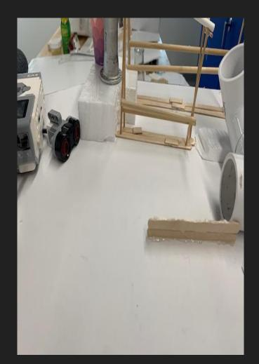
Step 4: The light gate detects the rolling marble and then activates a motor to move. The movement of the motor pushes a marble through a hole in the floor of level 1.
