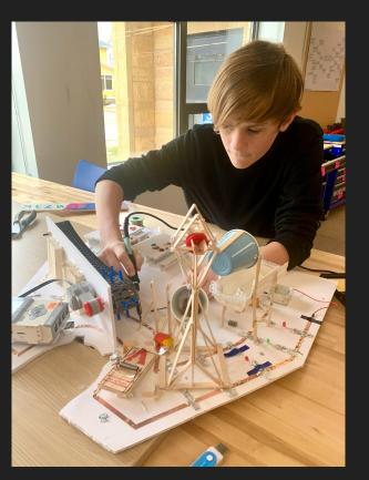
Zephyr is busy testing and soldering the 2n level LEDs
