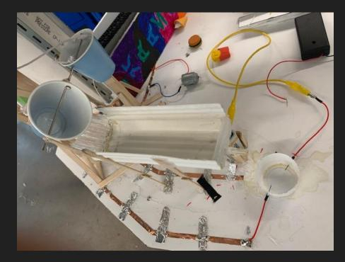
Step 10: The small cup will fill with electrolytic fluid, which will complete a small circuit and cause a small motor to turn.
