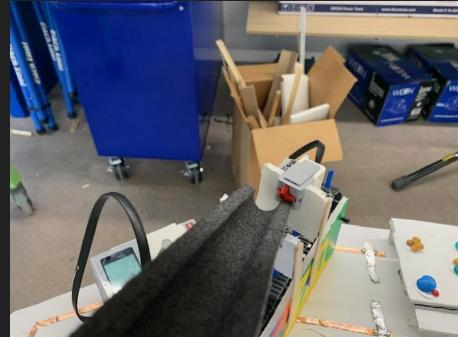
Step 6: When the marble touches the sensor, that activates the assembly line to bring food from one end to the other.
