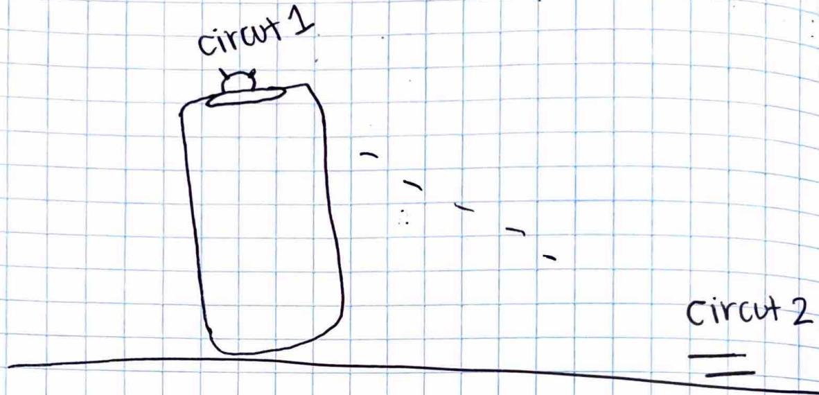
The clipboard is connected to two circuits. The first is when it is upright, it is connected to the clock motor. Once it falls it will disconnect causing the clock to stop moving. The second is after it falls, it will close a circuit that will start another motor.
