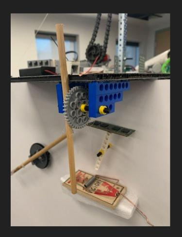
The rotating stick has copper foil tape on it and when it moves into its final resting position it connects a gap in the circuit to operate LED bulbs.
