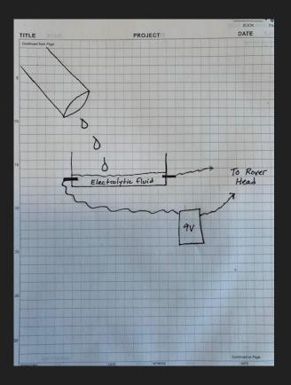
The presence of ions in the electrolytic solution allows current to flow from the battery to the LEDs that are inside the head
