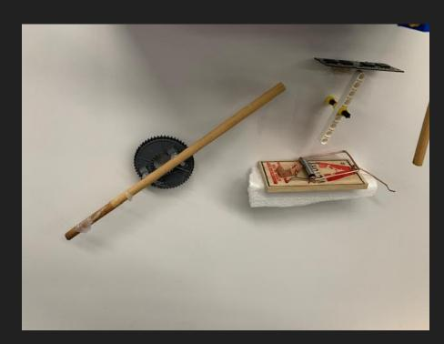
When it is triggered the mousetrap knocks a support out from underneath a small shelf
