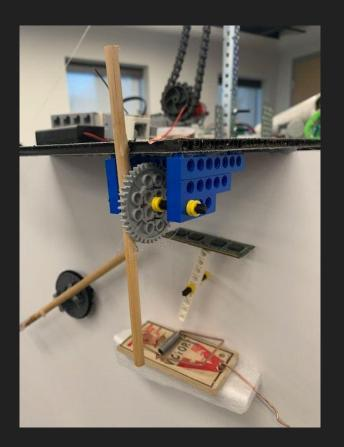
The shelf falls down and releases a weight that is attached to the end of a stick - the stick is attached to a rotating LEGO piece above it
