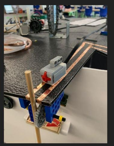
The stick also activated a touch sensor which signals the motor to begin the program.
