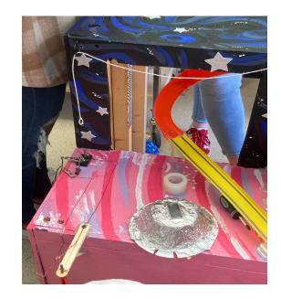
**Day 11: 1/25/23** Made a pulley system on the top of the tower that gets triggered when the ping pong ball hits the mousetrap. This hits the switch that turns on the electrical step.
