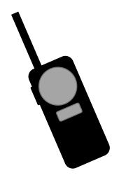
A two-way radio allows people to talk to one another over some distance by modulating and demodulating radio waves according to a signal produced by a microphone. These devices are used in commercial, government, and hobby settings.
